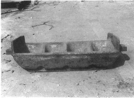
Figure 7 The ingot mould used for field tests.
